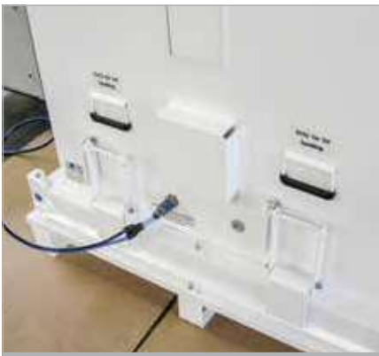
Water-vapour-proof container being leak-tested with overpressure
