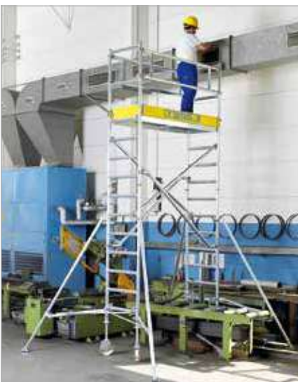
Brace-free mobile scaffold towers are available in two widths (0.75 m and 1.35 m), and they can be extended to heights of up to 10.40 m. Brace-free up to 1.90 m (middle).
