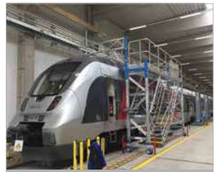
Single sided roof work platform with foldable railing cage for the maintenance of an Abellio train
