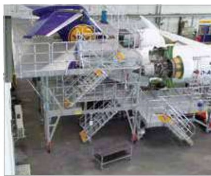
Height adjustable Tail- and enginedock for CRJ900
