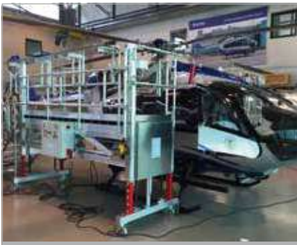
Maintenance platform with electrical height adjustment
