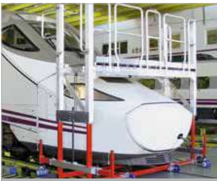
Height-adjustable front work platform with rail-guided chassis
